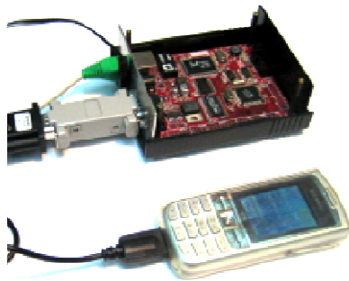
IMote2 (ZigBee communications, light and temperature sensors)
