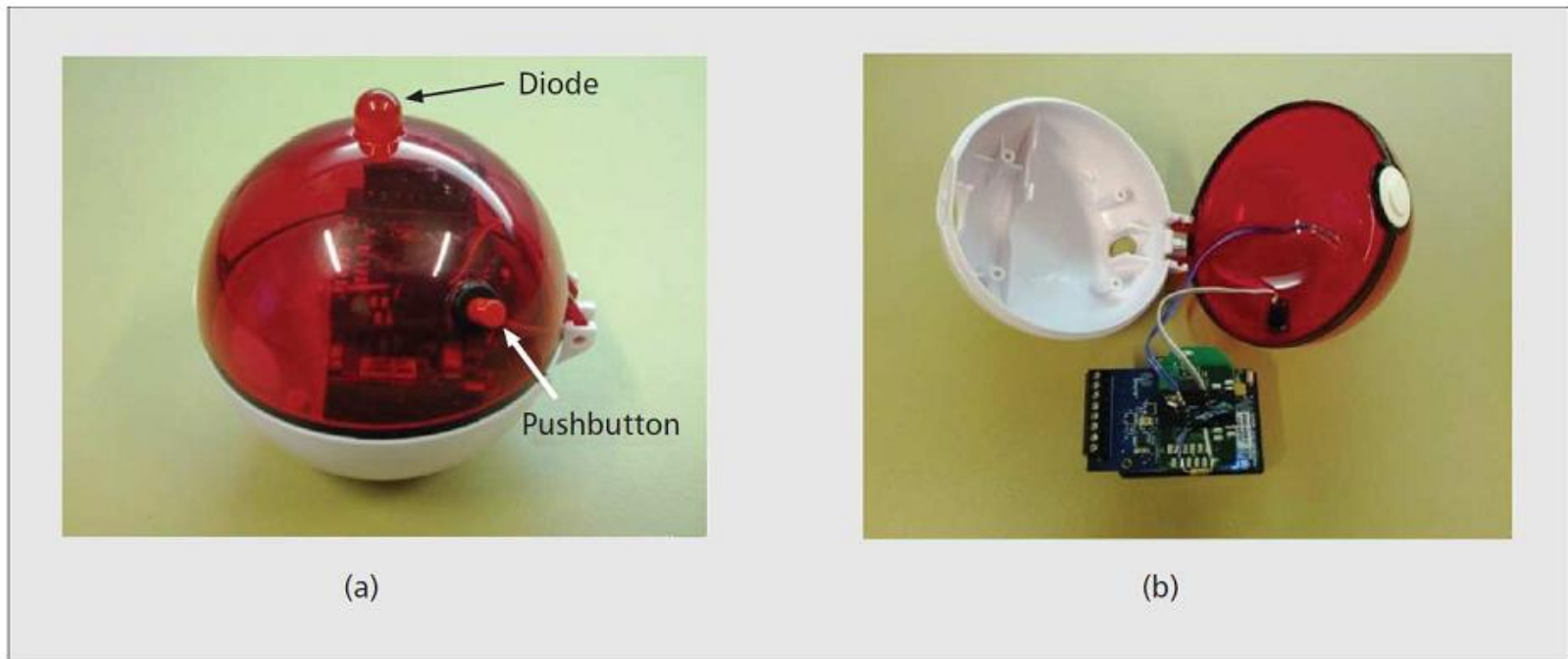
Figure 4. The POBICOS application pill: a) the user view: a pushbutton for starting/stopping the application, and a diode that shows the on/off status as well as the functionality level of the application; b) the internal view: the Imote2 (with the application binary and the POBICOS middleware) wired to the pill's button and diode.
